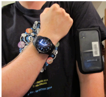
Figure 2: PulseCam prototype comprised of a LG G smart watch for continuously measuring one's heart rate and a Nexus S mobile device for capturing a picture. The Nexus S is situated on one's arm using an armband.
