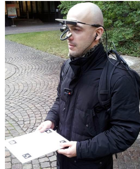
Figure 1. Mobile eye tracker (Ergoneers Dikablis Cable system) in action.
