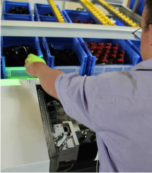
Figure 3: The position of the part that needs to be picked next is highlighted by the system.
