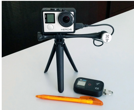
Figure 5: GoPro Hero 4 with an external directional microphone and a WiFi remote controller.
