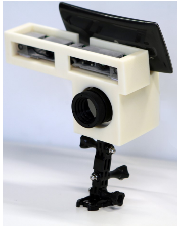
Figure 1: Hand Held prototype consisting of thermal, depth camera and a display for visualization.
